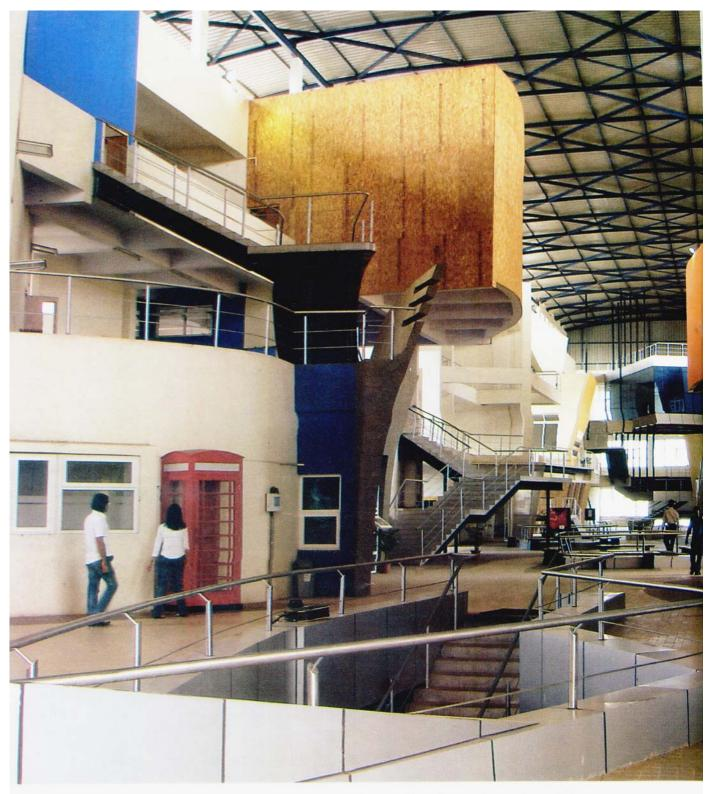
The amphitheatre overlooking the learning street is a hospitable space for hosting events. A huge steel truss anchored to the roof projecting on top of the street serves as the Prinicpal's cabin. With no columns on the street, the Principal's office on top allows free and easy pedestrian movement below.
